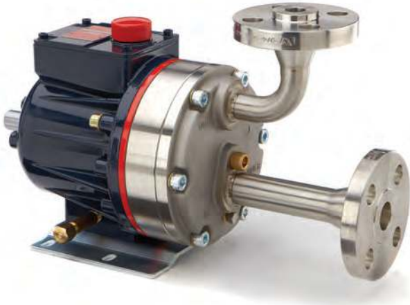
Model D10 (above left) fitted with ANSI flanges. Hydra-Cell pumps are also available with SAE or DIN flanges, NEMA or IEC motor mounts, or provided with ATEX certification to adapt to specific applications or meet international standards.
