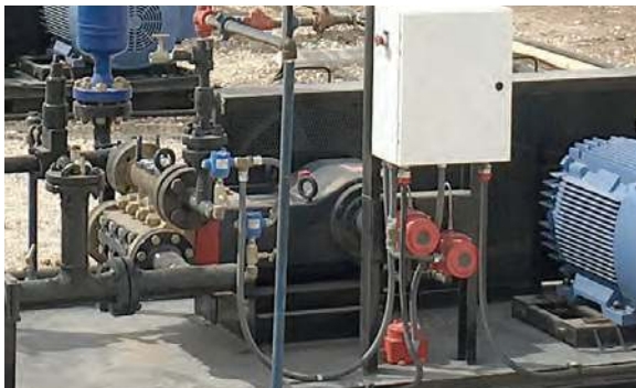
Hydra-Cell features a seal-less design that separates the liquid end from the hydraulic end, enabling the pump to tolerate solids, abrasives, and particulates, handle non-lubricating fluids, and run dry without damage to the pump.
