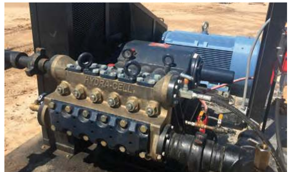
Hydra-Cell features a seal-less design that separates the liquid end from the hydraulic end, enabling the pump to tolerate solids, abrasives, and particulates, handle non-lubricating fluids, and run dry without damage to the pump.
