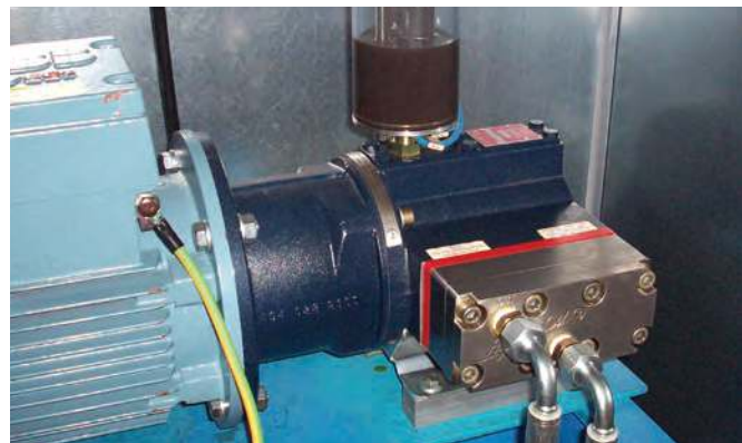
Hydra-Cell pump used in high-precision Pentane dosing. Hydra-Cell metering pumps can provide precise dosing at flow rates as low as 0.15 gph.
