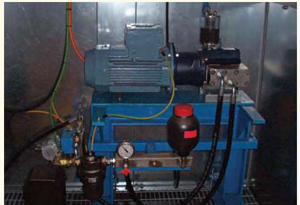
Pumping blowing agents requires a refrigeration unit. Significant capital savings are realized because space-saving Hydra-Cell pumps can be housed in a smaller refrigeration unit compared to pump types with the same flow and pressure ratings.
