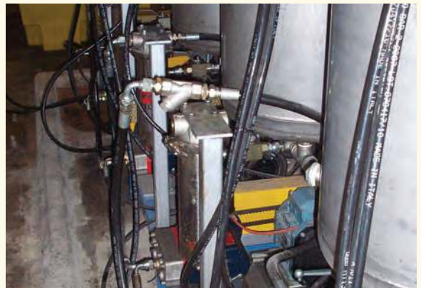
Injection of a proprietary catalyst into a high-volume polyurethane system. Where high flow is needed, Hydra-Cell pump models have maximum flow rates up to 66 gpm.
