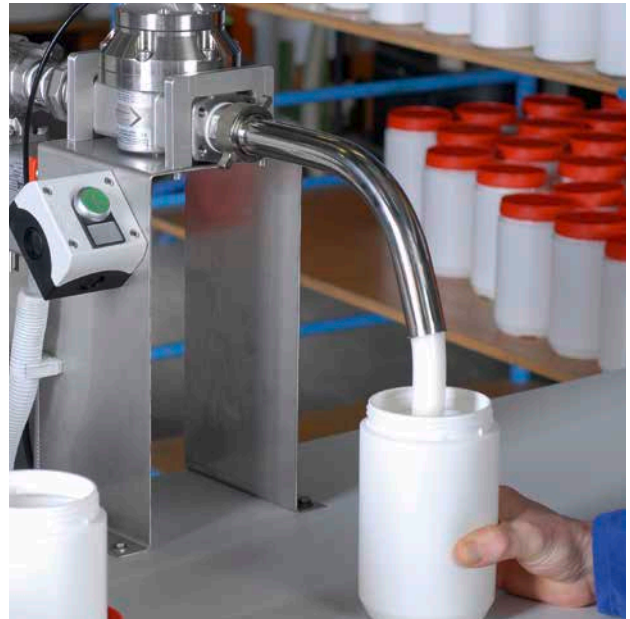
VISCOFLUX mobile – continuous transport using the example of vaseline.
