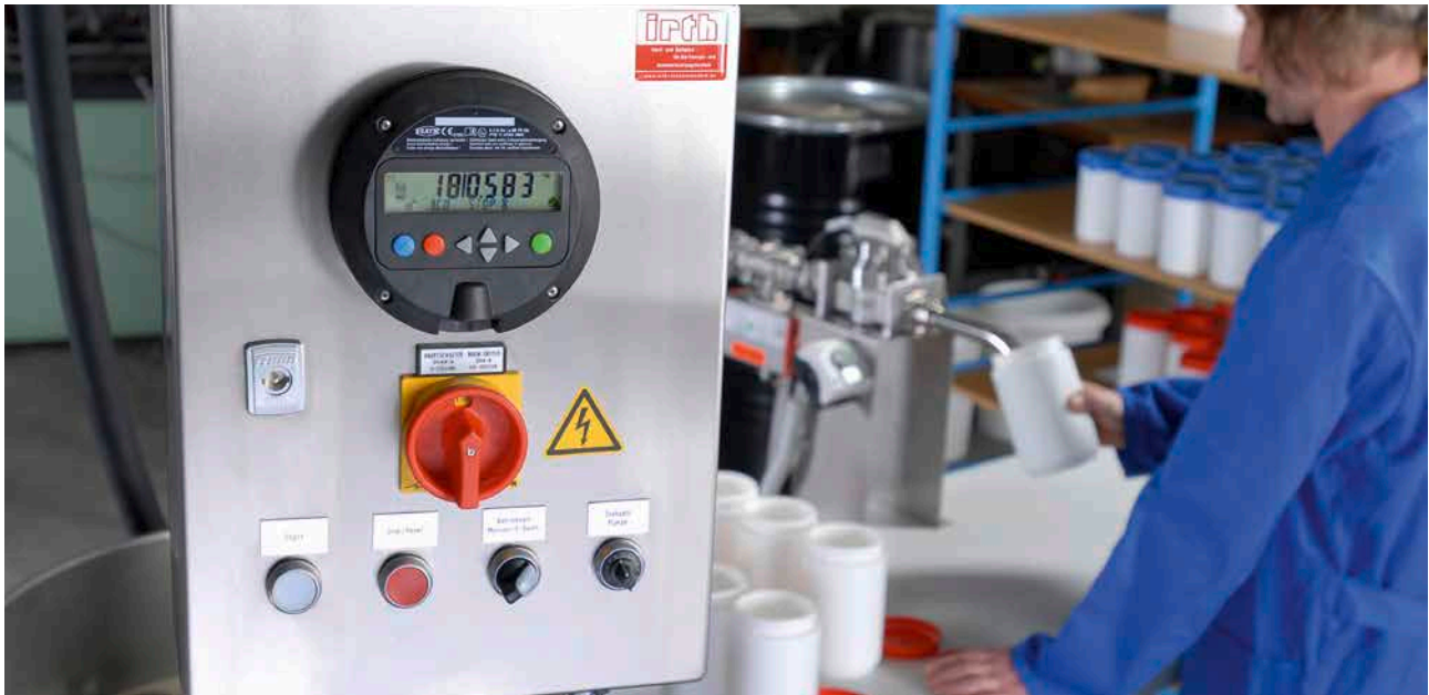
VISCOFLUX mobile – with control unit and integrated FLUXTRONIC® for use in batch processing.
