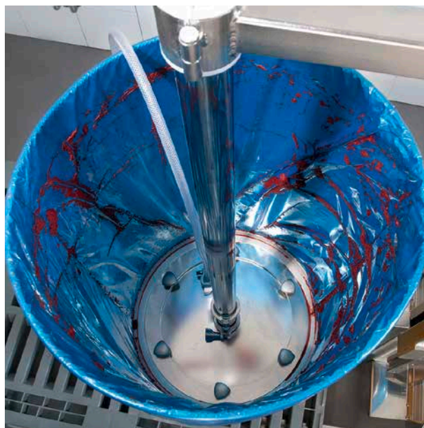
VISCOFLUX mobile – ideal for transfer out of conical drums with aseptic bags (example: tomato paste).
